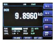
**D.C. Resistance Measurement**Ideal for inductive components'
